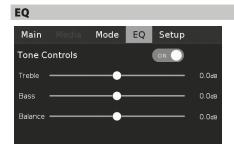
The M12 has the following Tone Control levels – Treble, Bass and Balance. Bass and Treble controls only affect the low bass and high treble leaving the critical midrange frequencies free of coloration. The Balance control adjusts the relative levels of the left and right speakers.
