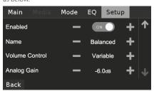
**Analog Gain:** -12dB to 12dB. Gain adjustment allows all sources to play back at the same volume level so you don't need to adjust the volume every time a new source is selected. It is generally preferable to reduce the level of the loudest source rather than making louder the softer sources.
